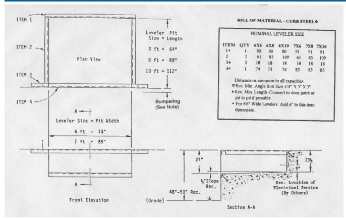
Note: Dock face and leveler protection req'd. Typical dock bumpers projection about 4" with level grade. Depressed drive surface can require additional bumper projection to protect building wall. Bumpers by others. Optional extra by Atlantic.
